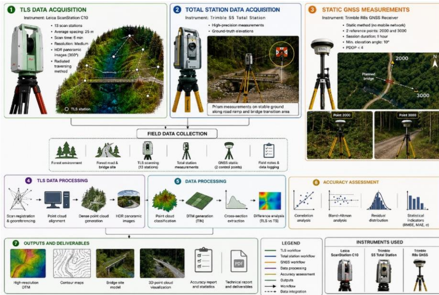
Figure 2. Integrated workflow for TLS, GNSS and TS data acquisition, processing and validation (Source: developed by the authors)
